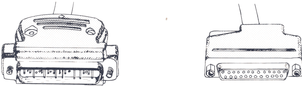
Figure A-1. 25-Pin Connector
